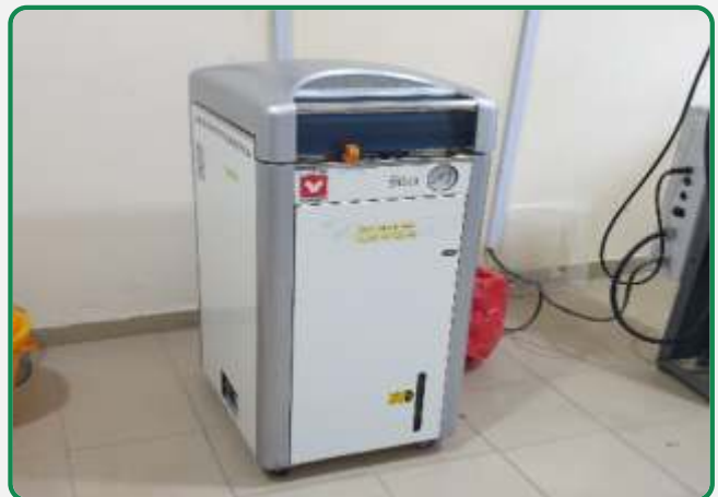
AN AUTOCLAVE MACHINE AT THE NATIONAL REFERENCE LAB. IN LAGOS (CPHL), USED FOR STERILISATION OF LAB EQUIPMENT
